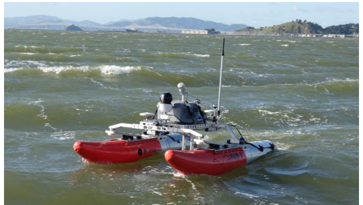
WAM-V 8 ASV for hydrographic survey
