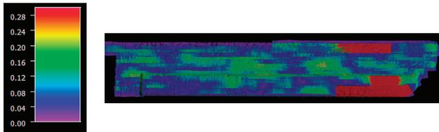
Using the same colour map, the equivalent surface is shown below, post-processed with the POSPac Go! SBET, and the improvement is clear.
