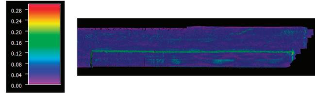
Note that the line of slightly higher standard deviation in the above POSPac Go! image is a result of the steep slope in the dredged area to the lower part of the image – see the bathymetric surface below.
